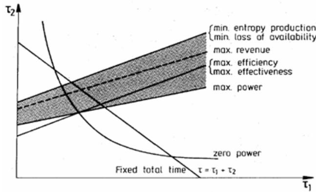
**FIGURE 3.** Time allocation on the hot/cold branch of an endoreversible engine for different objective functions.
