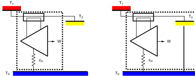
**FIGURE 7.** Heat engine supplied through a heat exchanger. The “system” is delimited by the dotted box. Optimizing the engine by itself (left) and including the exhaust reservoir (right) yield very different optima.
