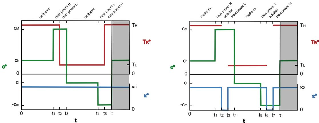
**FIGURE 5.** Optimal controls of the piston system when maximizing power output (left) and thermal efficiency (right).
