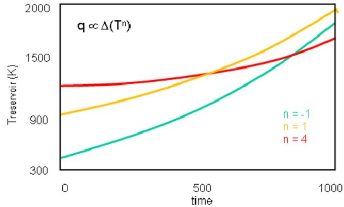
**FIGURE 8.** Optimal temperature paths for heating a system from 300 K to 900 K when the heat is transferred by thermodynamic force ( $n = -1$ ), by normal conduction ( $n = 1$ ), and by radiation ( $n = 4$ ).
