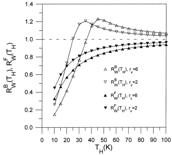
**FIGURE 9.** Work output per cycle for a Carnot engine using a Bose gas (open triangles), Fermi gas (filled triangles), and a classical gas (dashed line) as working fluid. (From [10])
