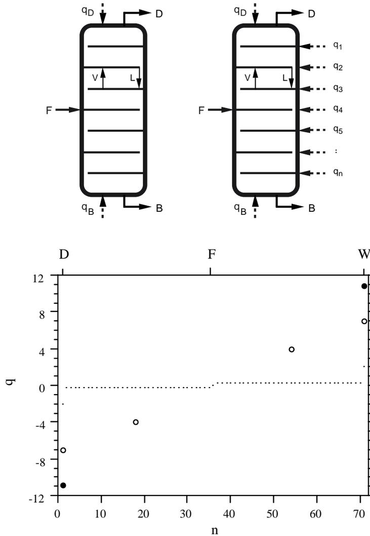
**FIGURE 6.** Conventional adiabatic distillation column (left) and diabatic column (right). Optimal rate of heat addition on each tray for a fully diabatic column (dots), for a conventional adiabatic column (2 solid circles), and for a column with just 2 additional heat exchange points (4 open circles) (lower frame).
