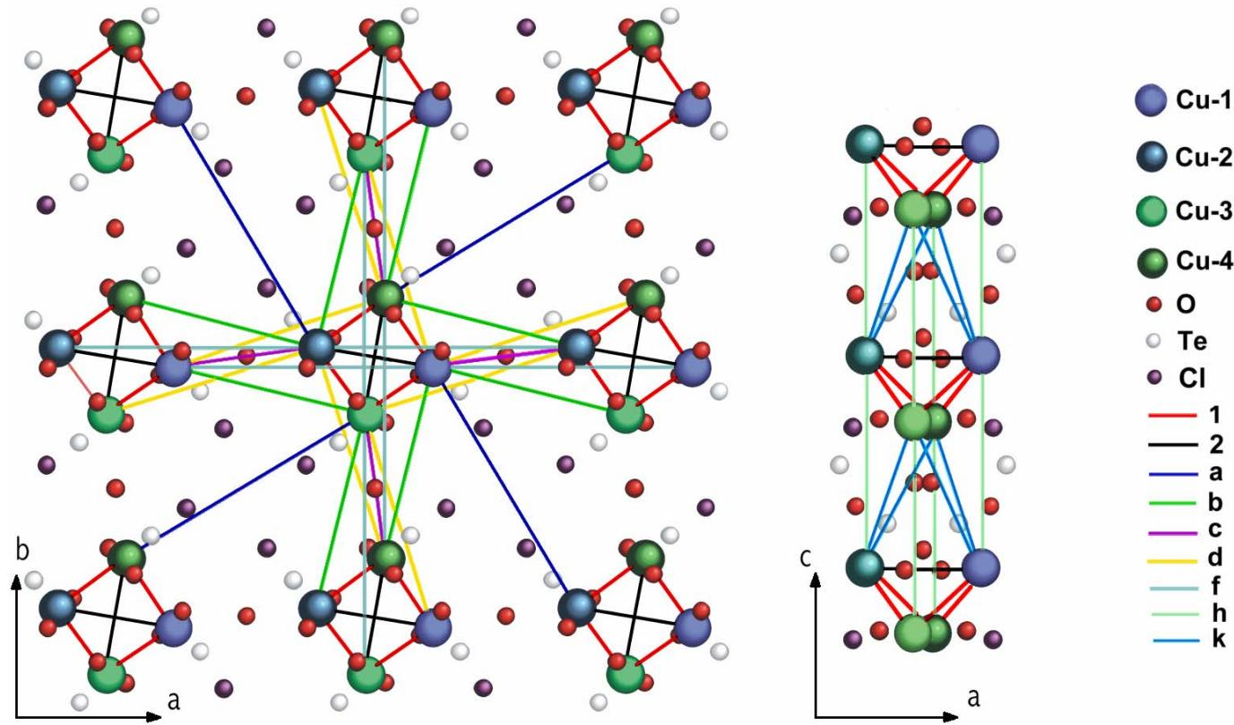
The  $\text{Cu}_2\text{Te}_2\text{O}_5\text{Cl}_2$  crystal projected on the  $ab$  and  $ac$  planes.
