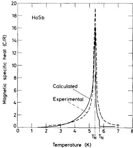
Fig. 2. The low-temperature specific heat of HoSb. The dashed curve shows the experimental results of Taub and Williamson [6]. The MF-result (solid line) exhibits a small jump at  $T_N$  (weak second-order transition) followed by a very strong, almost tricritical-like, peak at  $T'_N$ . The comparison is satisfactory, if it is assumed that the *small* peak expected experimentally at  $T_N$  is smeared out due to the strong one occurring at  $T'_N$ .
