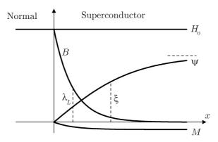
(a) To start with we consider the limit of  $\kappa \to 0$  or  $\lambda_L \ll \xi$ . Then B=0 for x>0 and according to (27.41) the wave function, which vanishes at x=0 and saturates at  $\Psi_0$  at large x, is
