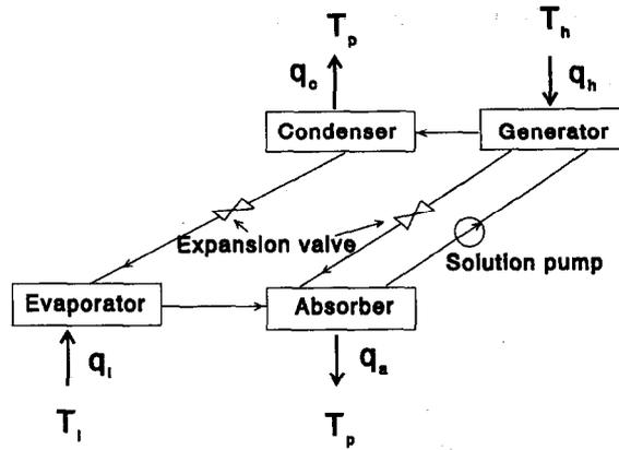
Fig. 1. An absorption heat pump system.
