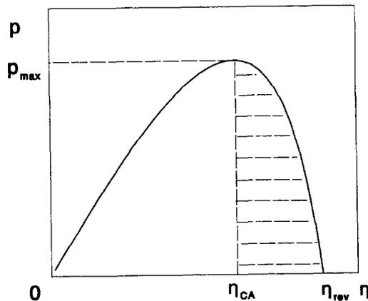
Fig. 4. The power output  $p$  vs the efficiency  $\eta$  for an endoreversible heat engine. The shaded region is the more efficient branch of operation for a given power production.
