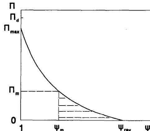
Fig. 3. The specific heating load  $\Pi$  vs the coefficient of performance  $\psi$  for an endoreversible absorption heat pump. Direct head conduction from the heat source to the heated space is marked as  $\Pi_d$ . The more efficient branch of operation of the driving heat engine is shaded.
