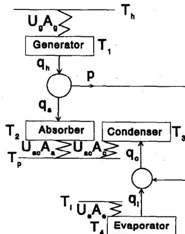
Fig. 2. The equivalent cycle model of an endoreversible absorption heat pump.
