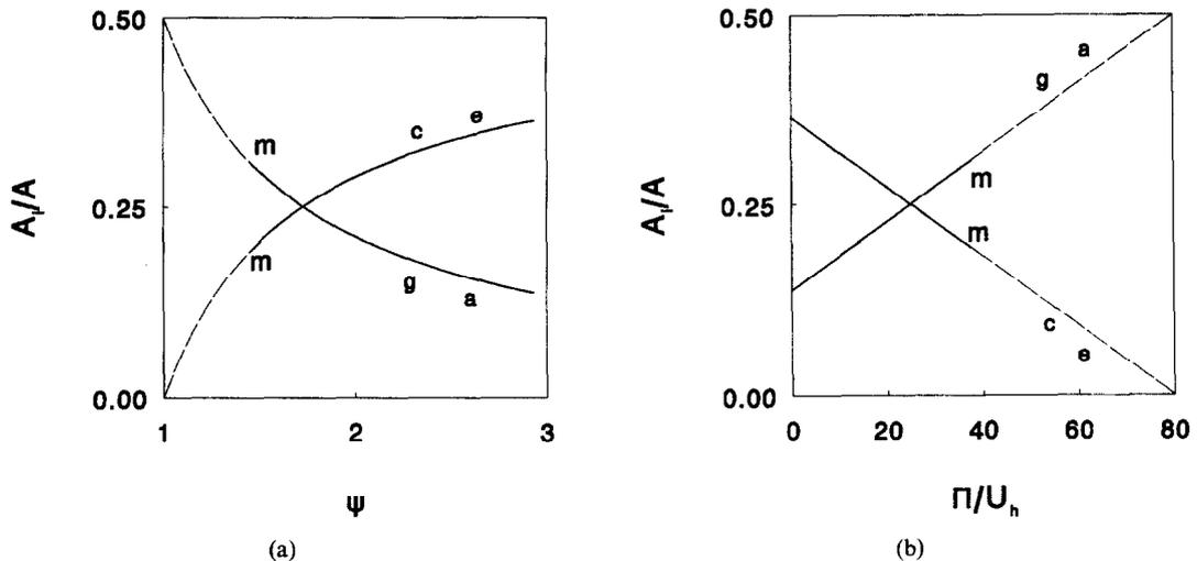
Fig. 6. The curves of the ratios of the heat transfer areas  $A_i/A$  ( $i = g, a, c, e$ ) vs (a) the coefficient of performance  $\psi$  and (b) the ratio of specific heating load to the heat transfer coefficient,  $\Pi/U_h$ , for equal heat transfer coefficients,  $\bar{U}_g = \bar{U}_{ac} = \bar{U}_e$ . The non-optimal regions are shown in dashed lines. The curves have been drawn for the temperatures  $T_h = 130^\circ\text{C}$ ,  $T_p = 50^\circ\text{C}$  and  $T_1 = 20^\circ\text{C}$ .
