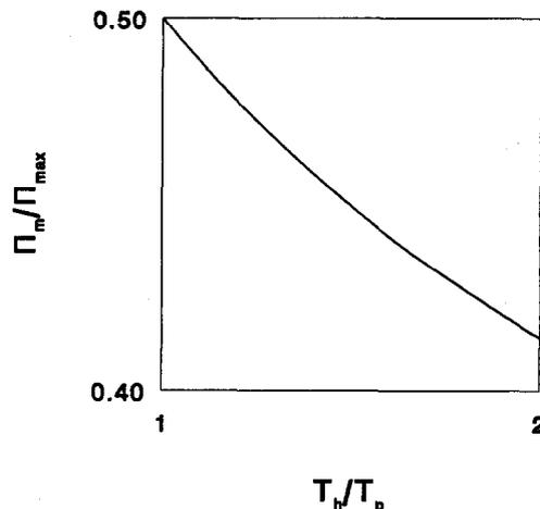
Fig. 5. The ratio of the specific heating loads  $\Pi_m/\Pi_{\max}$  vs the ratio of the reservoir temperatures  $T_h/T_p$  for an endoreversible absorption heat pump with  $U_h = U_p$ .
