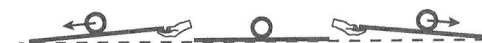
Figure 2. An illustration of the energetics along a neutral degree of freedom: the horizontal table. Note that only a very small elevation suffices to make the process go in one direction or the other.
