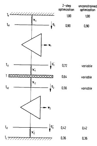
FIG. 1. Two staged CA engines. In the numerical examples  $T_H$  and  $T_L$  are the same as in Fig. 2. The first column results from the staging of two individually optimized CA engines with the intermediate temperature T a constant. The second column results from an unconstrained optimization of the whole system.
