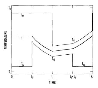
FIG. 3. Temperature sequence during one period for the system shown in Fig. 1 resulting from unconstrained optimization, i.e., corresponding to the last column of Fig. 1.
