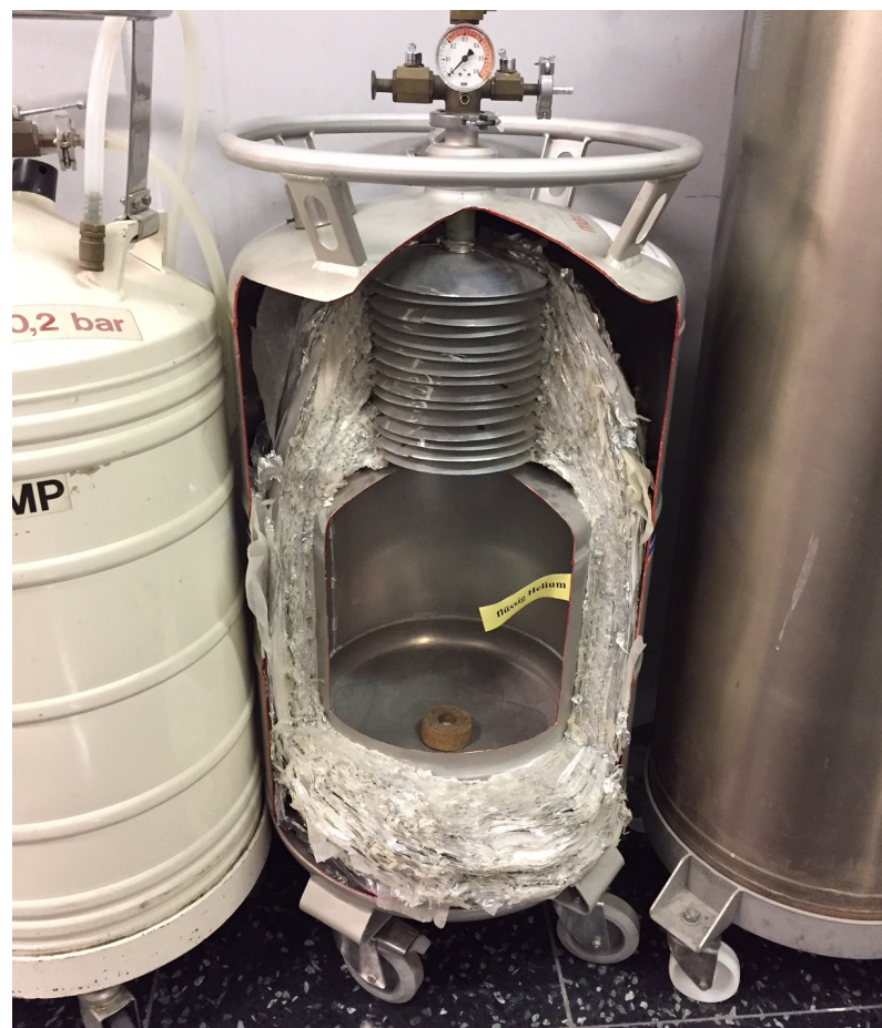
Figure 5. This liquid helium container minimizes the rate of heat leaking in by forcing literally hundreds of small equilibrations along the way.
